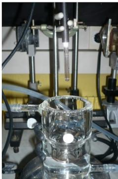
**Fig. II.3.** Pyrex cylindrical photo-reactor
